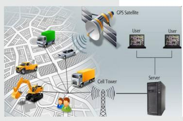
Live Fleet Monitoring System is a GPS based tracking system that provides Internet-based access to LIVE vehicle tracking and asset management. Knowing where your vehicles and assets are at all times gives you the power to make time and money-saving decisions with a quick glance.
